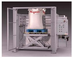
Stainless Steel Bulk Bag Conditioner with programmable scissor lift and automated turntable raises, lowers and rotates the bag in any degree for complete conditioning on all sides at all heights.
